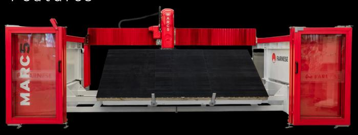
The MARC5 from Farnese marks a significant entry into the realm of fully CNC-controlled 5-axis bridge saws. It combines an onboard CNC controller with user-friendly software, making it one of the most versatile and accessible machines available, a true hallmark of the Farnese brand.
